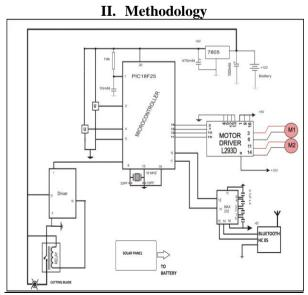
Figure1: Block Diagram of solar powered automatic lawn mower
